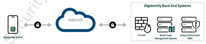
Digidentity has no access to the contents of the VSC. The user has sole control over the cryptographic keys on the VSC. The Digidentity VSC is patented (number EP2414983A1).
